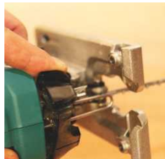
▲ The blade is ejected using the plastic front lever
